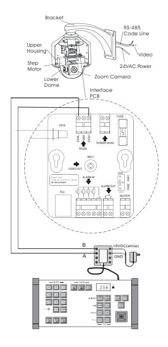
NOTE: To connect RS-485 code line to SECUPRO matrix system, Be sure to connect DATA- to A, DATA+ to B. For other system, if it doesn't work, connect A to B, B to A.
