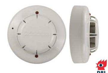
The Fyreye Extra optical smoke detector uses a pulsing IR LED & photodiode to detect IR scatter caused by smoke entering the chamber.
