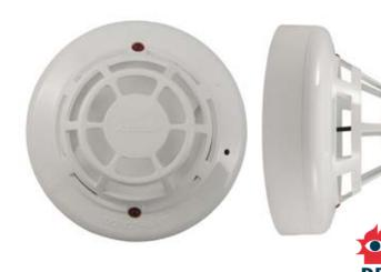
The Fyreye Rate of Rise heat detector (FEHE2000) uses a thermistor arrangement to sense a quick rise in temperature and also a final threshold temperature of 57°C. The Fyreye fixed heat detector (FEFHE2000) has a single thermistor arrangement that gives an alarm at a temperature of 90°C.
