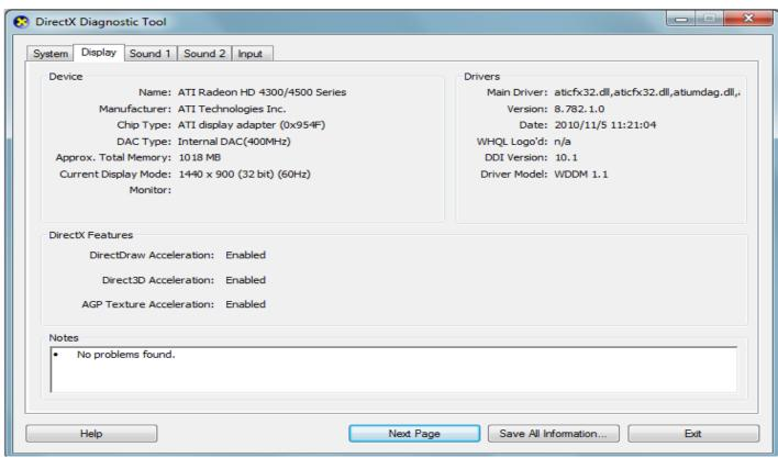
If the DirectX is 【DirectDraw Acceleration: UNABLE】, it means you didn't install the graphic card driver, or installed incorrect. Please install graphic card driver again.
