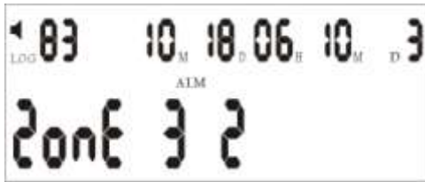
Figure18: The LCD display when the wireless detector is alarming
