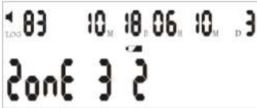
Figure 25: Detector No 2 in zone 3 is low voltage
