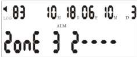
Figure19: The LCD display when the wired detector is alarming
