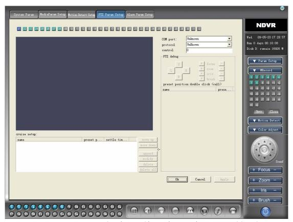
Process PTZ parameters set to begin confirmation equipment used by the right agreement, supporting baud rate, and used by the serial port,PTZ decoder addresses. After confirmation on the above information can be setting.
