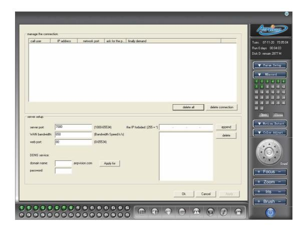
Server Ports: defaults to 7000, when remote users connect to the port of importation, if multiple mainframe recommended choice to 256 for the port spacing, such as 7000,7256, and so on.
