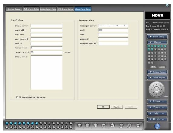
Including mail messages warning alarm parameters and parameter settings, installed after completion of parameters can be set up in the media and in the opening movement set up to detect the function, trigger conditions including video loss, object movement, IO alarm etc.
